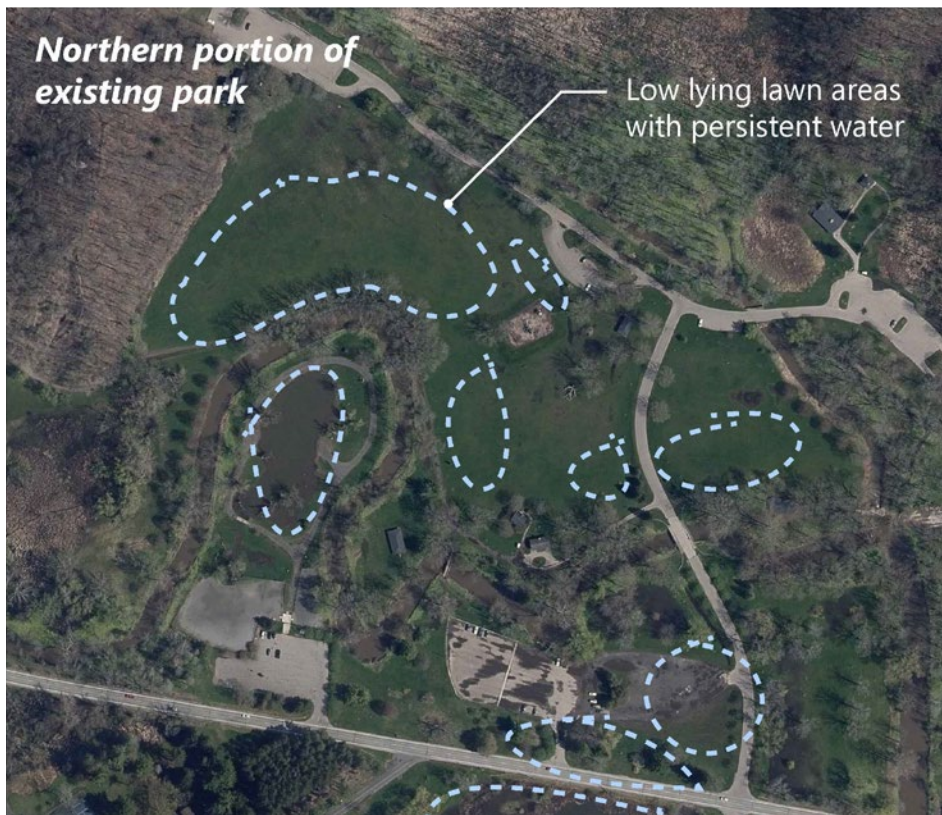
Existing conditions and aerial photo of northern area of Ellison Park. Indicated areas observed to be consistently wet 4 to 5 days after modest rain events.
